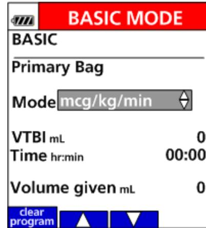
Figure 34. Arrow Soft Keys used to scroll through Dose Rates
