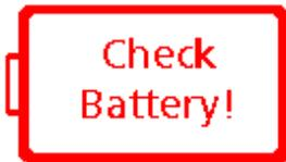
Battery Error. An error code number may also be displayed. Refer to the Service Manual for a description of the error code. (red battery)
