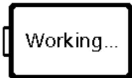
Initial pump screen when AC power is supplied and the pump is powered off. Battery charger is determining the current status of the installed battery. (black battery)
