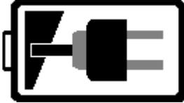
The AC adaptor is connected and the Wireless Battery Module is being charged. Battery segments (bars) indicate battery charge level. (black battery; white background)
