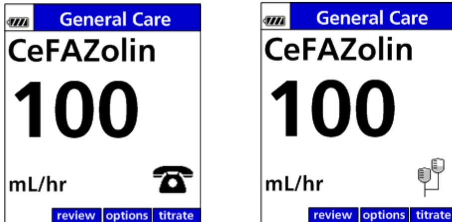
Figure 49. Alternating Run Screens with Secondary Callback Enabled.
