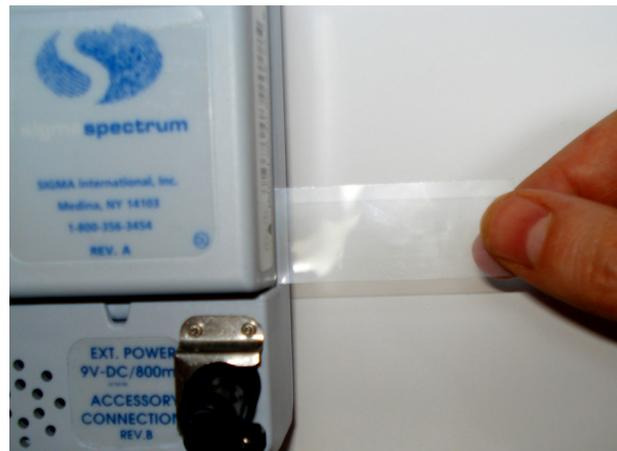
Figure 7. Battery Tab.
